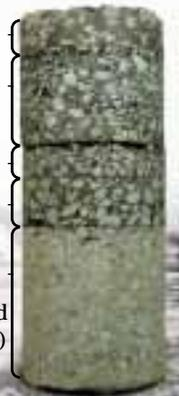
Core from a resurfaced road (A39)
