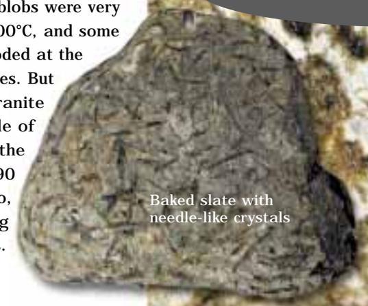
Baked slate with needle-like crystals
